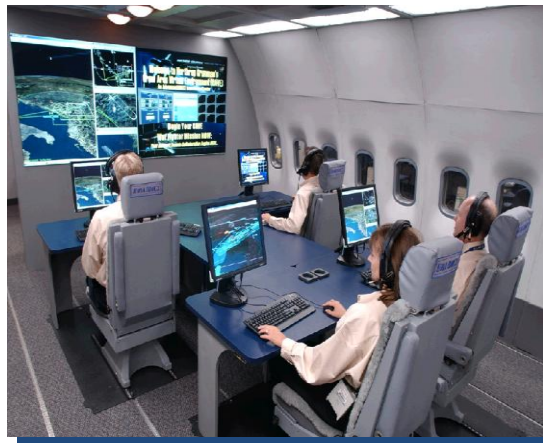
Figure 3-8. Conceptual arrangement of the BMC2 suite of the E-10A 6
