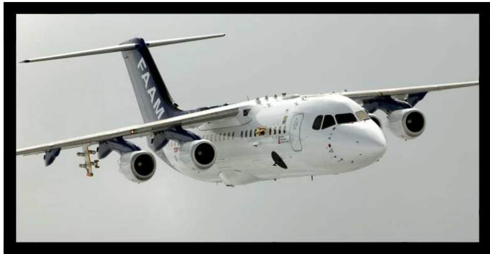
Figure 3.1: The Facility for Airborne Atmospheric Measurement (FAAM) aircraft. The BAe-146 is equipped with high quality instrumentation, capable of recording high frequency measurements of temperature, humidity and three dimensional winds, amongst other variables.
