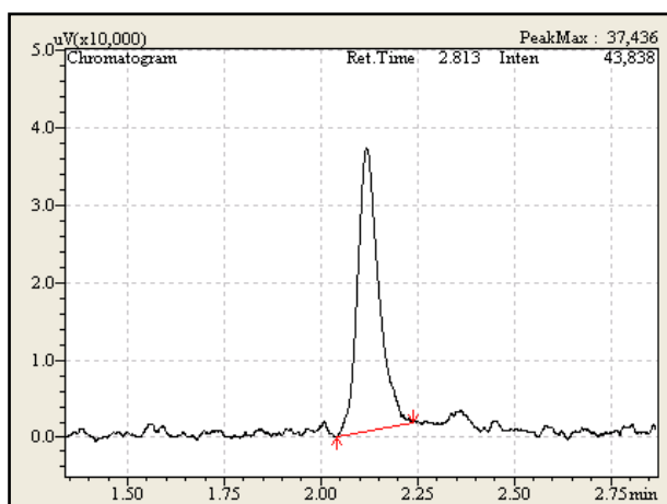
Figure 2.7 Example of GC chromatogram for a DMSP sample. The peak has a Retention Time (RT) of 2.05 min and the peak area is automatically integrated by the software (delimited by the red line and arrows).
