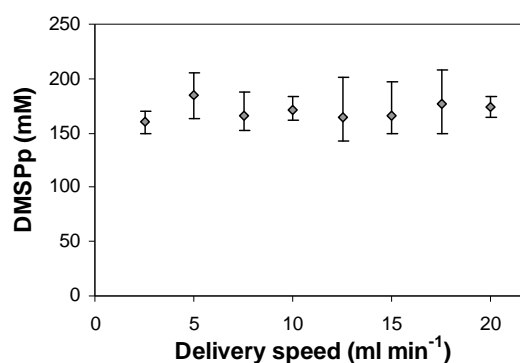
Figure 3.11 Effect of 8 delivery speeds of the syringe pump on the \text{DMSP}_p values using the 10 ml syringes and 2 ml culture sample of Heterocapsa triquetra culture at 3 \times 10^4 \text{ cell ml}^{-1} . Shown are average values with ranges of data ( n=3 except n=2 for 2.5 and 5 \text{ml min}^{-1} ).
