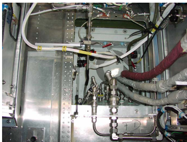
Fig. 6. Photo of the container connector bracket viewed through the cutout in the container floor. The aerosol tube is on the left (with short black flexible section). On the right the insulation of the 3 heated tubes is visible. The exhaust tube is in the centre. The non reactive trace gas tube is to its left. The 3 electrical power and data connectors are black. Also visible is the dark green sleeve of the optical fiber cables in the upper right corner. Altogether 12 connections between container and aircraft are involved plus an electrical bonding lead.
