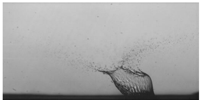
Figures 5 a (free surface simulation) & b (experiment). 70° impact of a 483x170 \mu m droplet at 55m/s over a 50 \mu m water film thickness and at ambient temperature.
