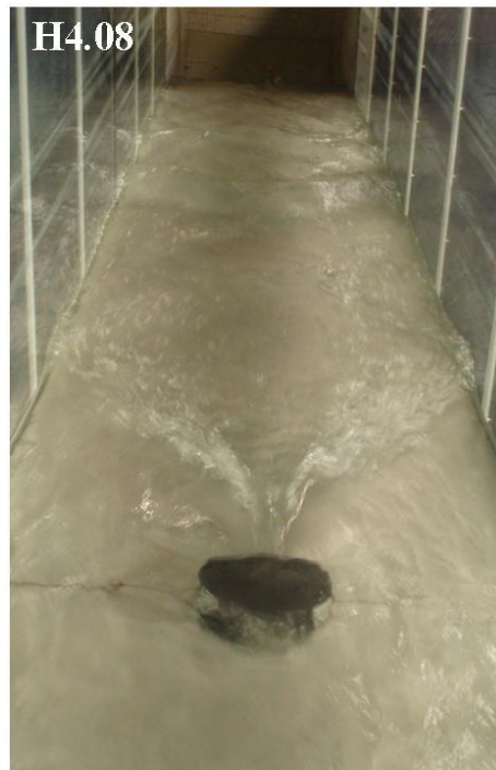
Figure 3.10 Oblique views of flow fields from a few tens of centimetres upstream of the hemisphere to the downstream end of the flume, from Series H4. From photograph A – D the flume pumping rate increases. Flow became supercritical as it travelled around or over the hemisphere and the pattern of hydraulic jumps varied with the Froude condition of flow upstream of the hemisphere (marked on the overlay). In (A) and (B) the flow did not overtop the hemisphere. Hydraulic jumps were straight-fronted and oblique to the main flow direction (Shape II, Table 1.1) Note how the fronts of the flow-parallel hydraulic jumps closed from (A) to (B) and then widened from (B) to (C) as the hemisphere was overtopped by flow. In (C) the hydraulic jump has an arcuate front (Shape V, Table 1.1). Between (C) to (D) the hydraulic jump has transformed into the arcs of overturning water (Shape VIII, Table 1.1).
