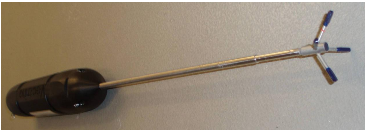
Figure 2.5 A Nortek Vectrino + acoustic Doppler velocimeter. The black casing houses the circuit boards. The 0.008 m diameter stem joins the circuit boards to the probe head, which has five blue parts that emit and sense acoustic signals.
