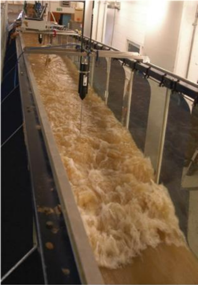
Figure 4.8 Oblique photograph of the water surface of the supercritical flow, hydraulic jump and tailwater in Run 2.
