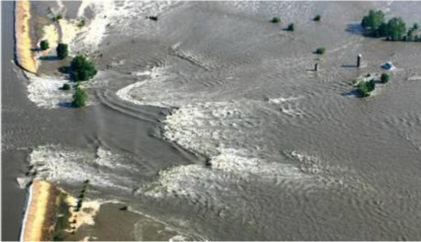
Figure 1.10 Flow becoming supercritical as it passes over a levee of the Mississippi river. Photograph sourced from http://lassiegethelp.blogspot.com/2008/06/lawless-stream.html and has been released into the public domain.
