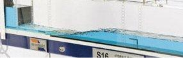
Figure 1.9 Flow becoming supercritical as it passes under an undershot sluice gate in an Armfield sediment demonstration flume. Reproduced with permission of Armfield.
