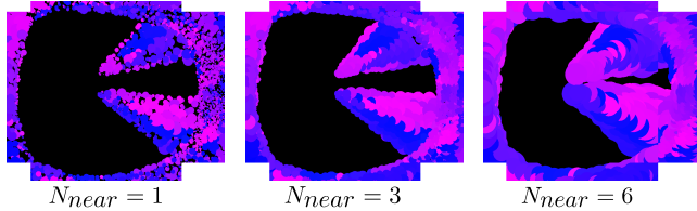
Figure 12: Effects of varying the parameter N_{near} on point splatting: too small a value (1) creates holes, while too large a value (6) results in redundant overlapping splats. We use N_{near} = 3
