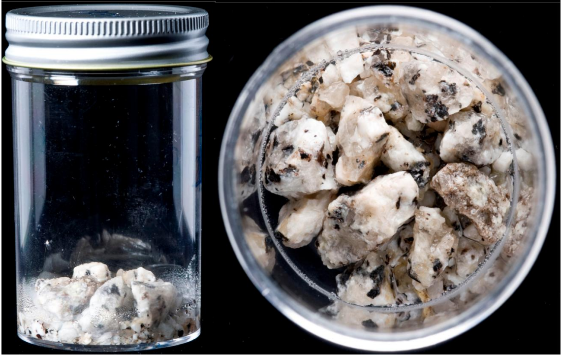
Figure 4.1 – Side and plan views of a granite control microcosm (after a weathering period of 113 days). NB the black flecks in the granite clasts which are the mineral biotite. Condensation on the walls of the jar was removed using swabs and a hairdryer prior to photographing.
