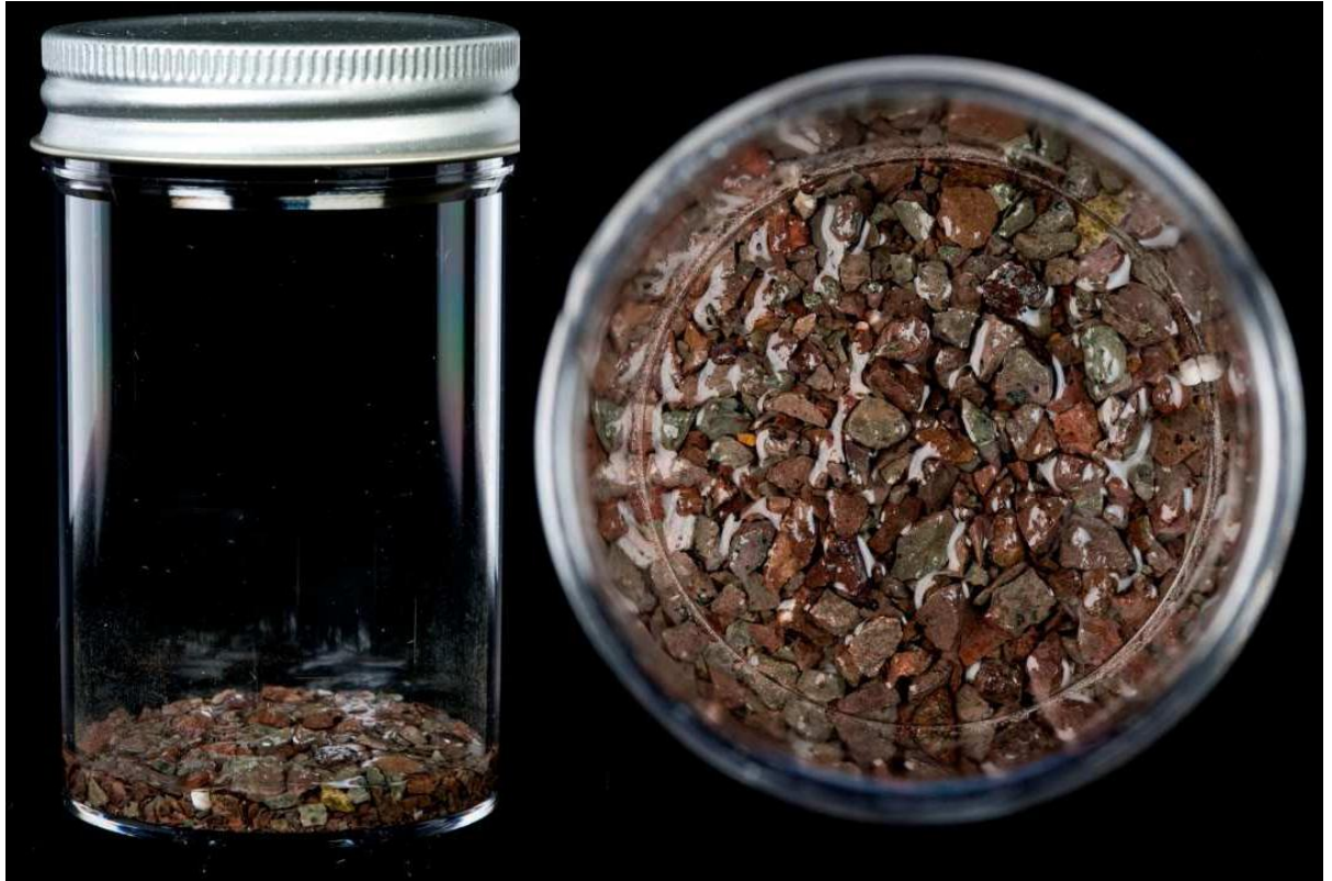
Figure 4.9 – Side and plan views of an andesite control microcosm shortly after preparation.
