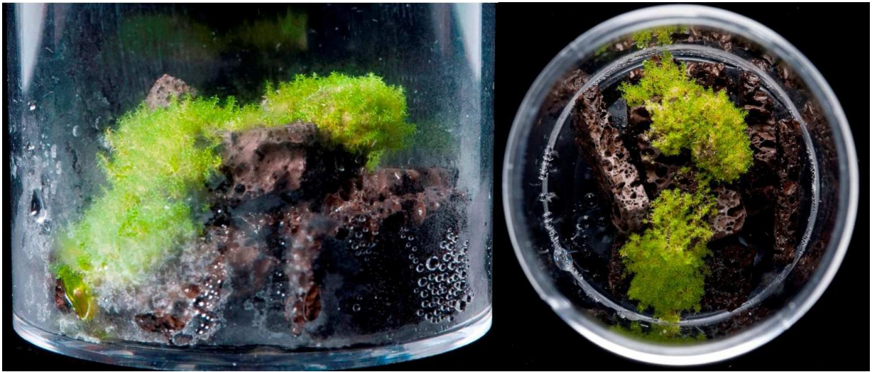
Figure 1.6 - Side and plan views of a Basalt microcosm (after a weathering period of 138 days).
