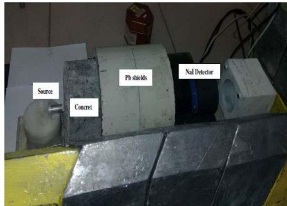
Fig. 3. Image of the radiation test by gamma source and counting by the NaI (TI) detector.
