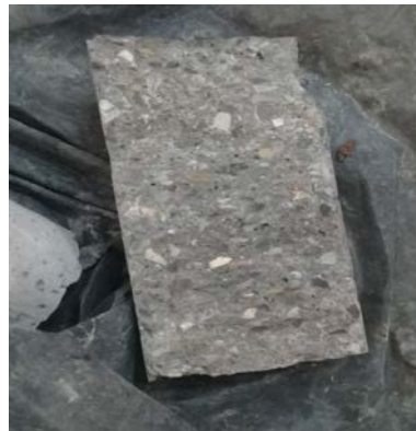
Fig. 6. Splitting sample image of Brazilian test
