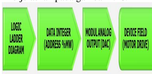
Gambar 4.4 Alur proses sinyal analog output
