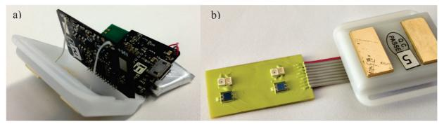
Fig. 1: a) Probe for measuring biosignal form BioSense system. b) Modified probe with integrated pulse oximetry on extension board.
