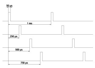
Fig. 4: LED switching timing diagram.
