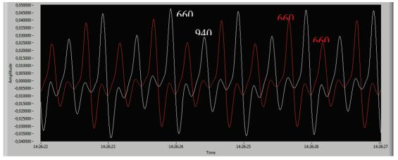
*Fig. 3: Signal from both sensors, shows dependence of the wavelength of used light.*
