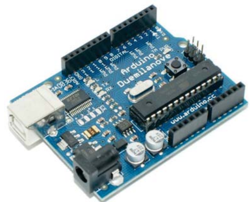
Fig. 3: Development board Arduino Duemilanove with microcontroller ATmega328P.
