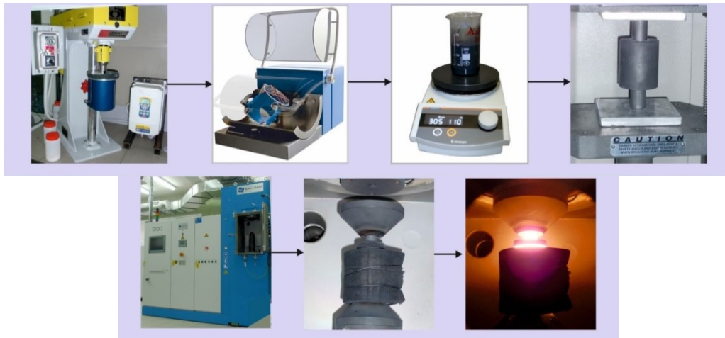
FIGURE 1. Scheme of creation technology of cutting ceramic sample: refinement powders (wet grinding), evaporation, pressing, sintering [5].
