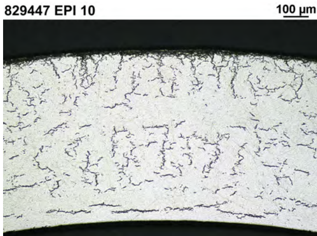
FIGURE 12. Sample 829 447. After hydrogen charging with inner pressure 3 MPa.
