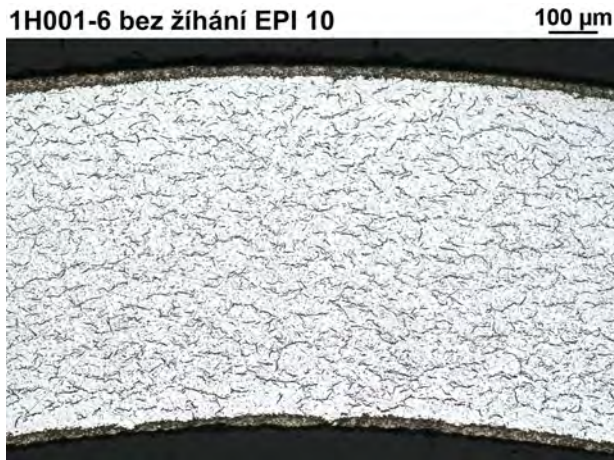
FIGURE 7. Sample 1H001, section 6. Prepared after hydrogen charging (without annealing).
