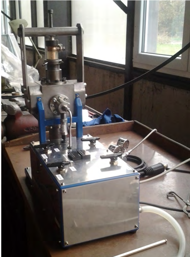
FIGURE 1. Device used for-welding samples.
