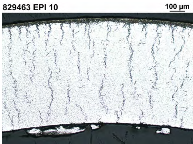
FIGURE 13. Sample 829 463. After hydrogen charging with inner pressure 9 MPa.
