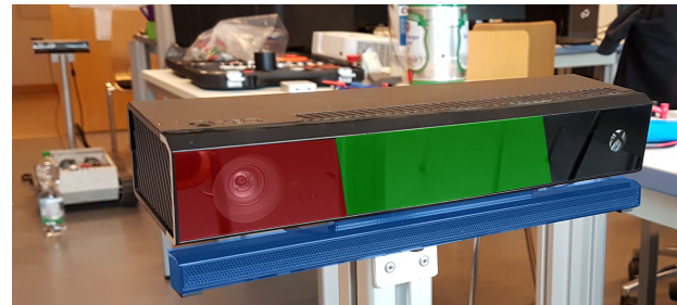
FIGURE 2. Overview of the Kinect camera.
