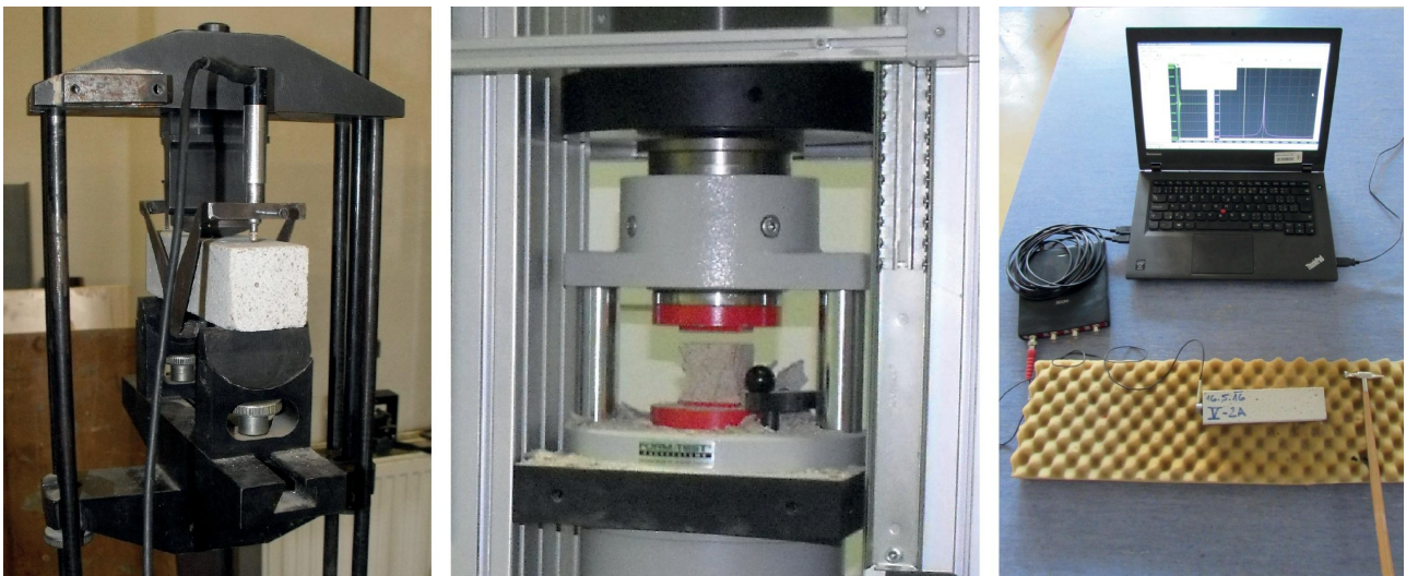
FIGURE 2. Arrangement of the fracture test (left), compressive strength test (middle) and resonance test (right).
