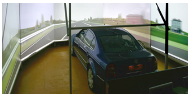
FIGURE 1. Advanced driver simulator for driver drowsiness research.
