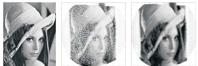
Fig. 10: 2-D Scan (left: original image, middle: sampled image, right: interpolation)
