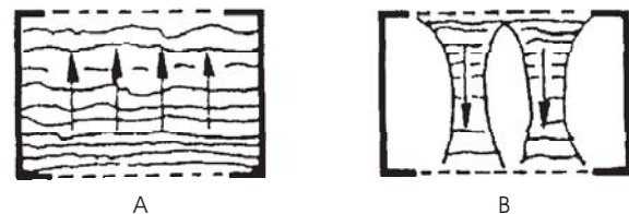
Fig. 5: Cold air inlet location for room cooling (A correct, B incorrect, because the falling cold air streams are constricted)
