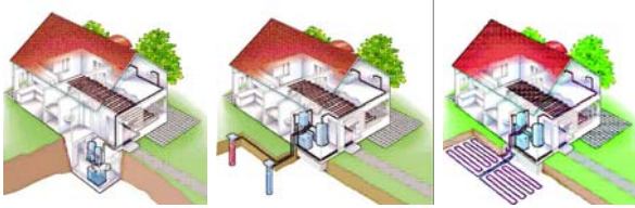
Fig. 2: Air, water, soil to water heat pumps [*2]
