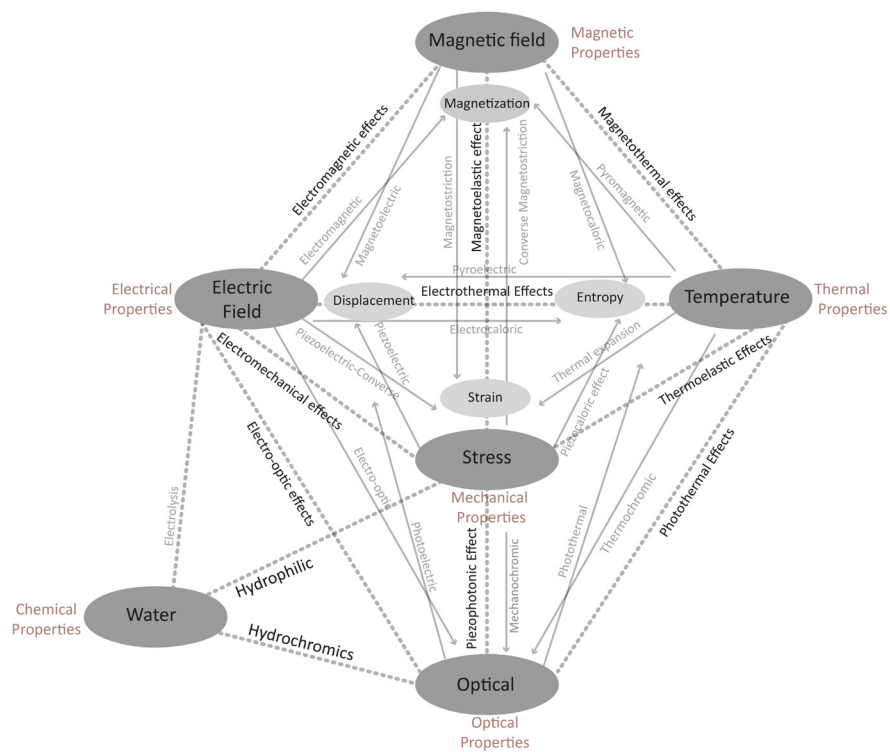
FIG. 1 Diagram characterising the behaviour of smart materials. Based on the Heckman Diagram
