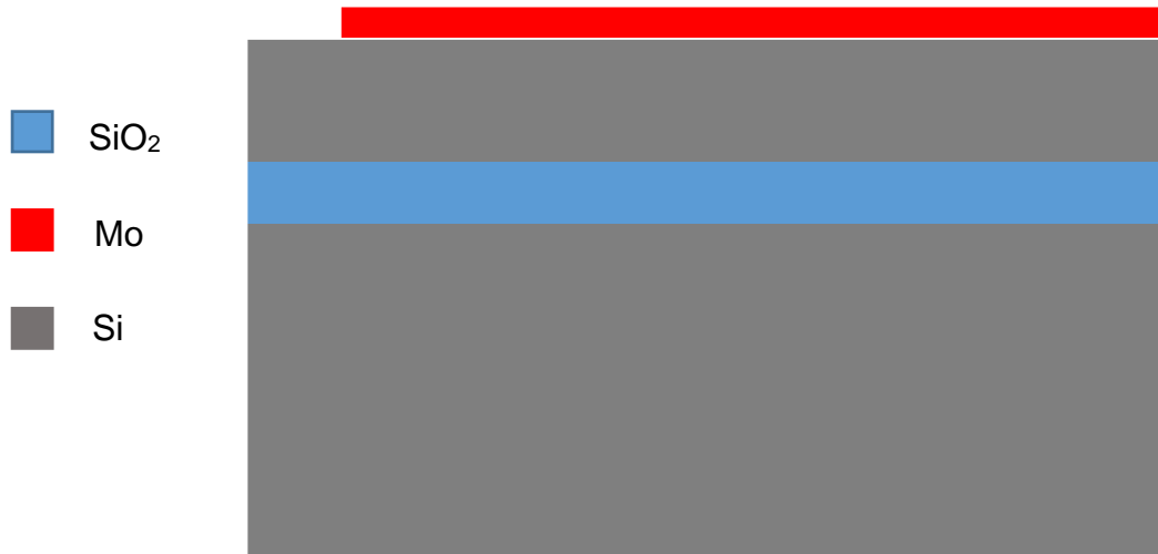
Figure 6. The bottom metal deposition and patterning. Molybdenum is the material of choice for bottom metal.
