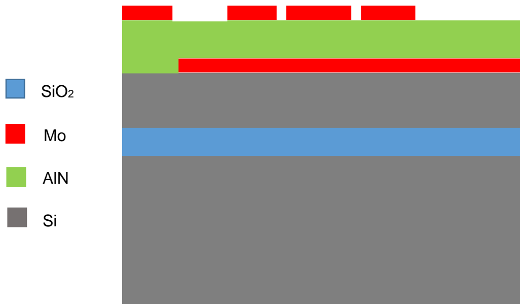
Figure 8. The top metal Mo sputtered on the AlN and then patterned to create top electrodes and contact pads.
