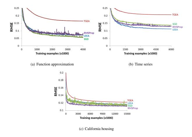
Figure 3.1: **Average root mean square error on the test set over time.** The average performance over total training examples seen so far as measured against the test set is displayed for each algorithm on the (a) function approximation, (b) time series, and (c) California housing domains. The main result is that the performance of LEEA closely matches that of SGD and RMSProp.
