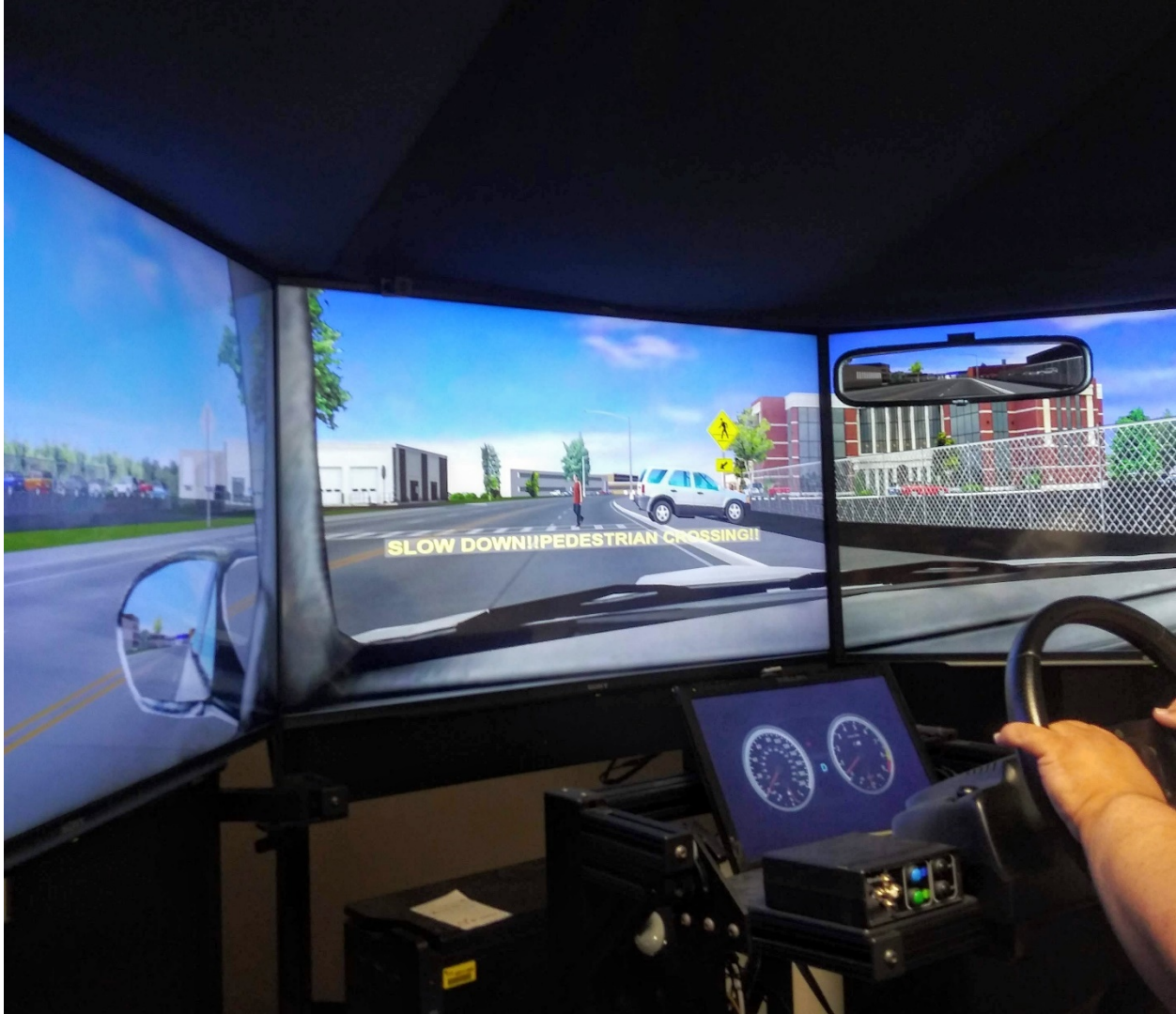
Figure 12. NADS MiniSIM driving simulator with HUD interface
