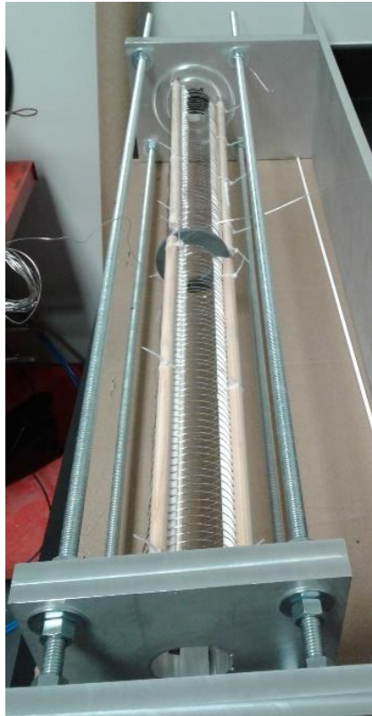
Figure 65. Heater assembly during construction
