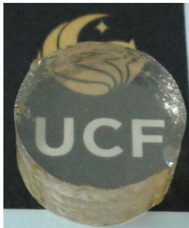
Figure 12. 70\text{TeO}_2\text{-}20\text{WO}_3\text{-}10\text{La}_2\text{O}_3 melt/quench sample
