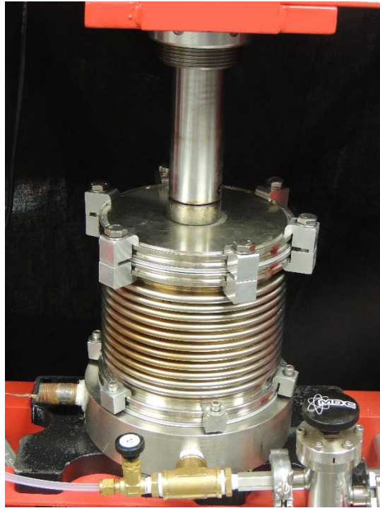
Figure 18. Vacuum capable sintering vessel
