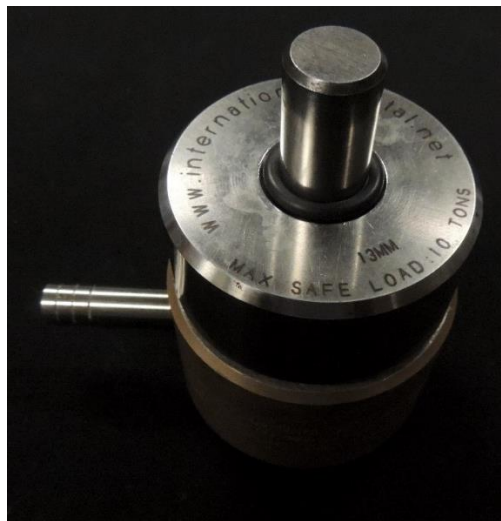
Figure 14. 13 mm diameter vacuum capable die used for cold pressing
