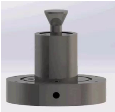
Figure 10. Representation of resistive heater surrounding a uniaxial steel die
