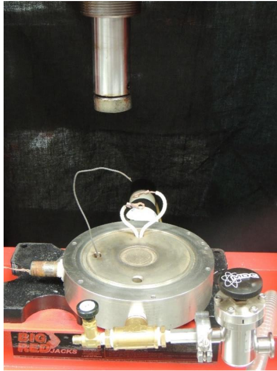
Figure 17. Base of the vacuum capable sintering vessel
