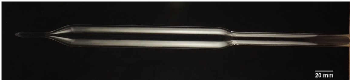
Figure 67. Growth ampoule is 20 mm inner diameter (ID), 24 mm outer diameter (OD) by 200 mm length with a 3 mm ID by 6 mm OD by 35 mm length capillary making up one end. The other end of the ampoule is a 10 mm ID by 14 mm OD by 150 mm long section meant to connect to existing vacuum valves.
