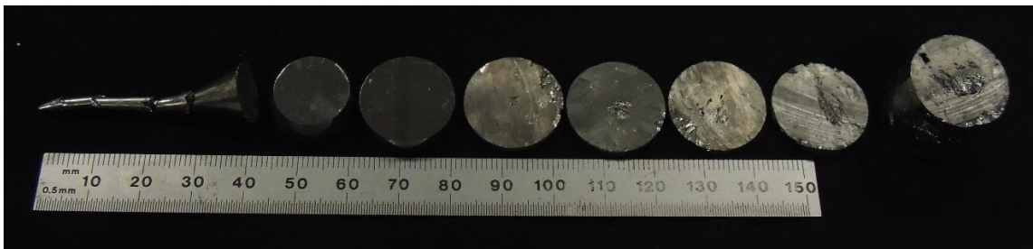
Figure 73. Tellurium crystal boule cut into slices
