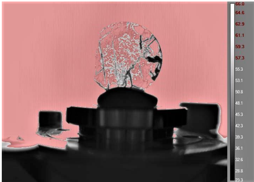
Figure 83. Tellurium slice seen in transmission using an infrared camera
