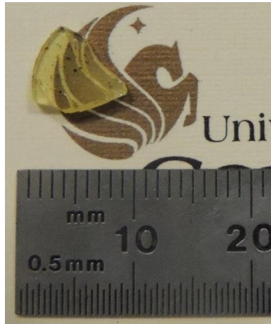
Figure 42. A piece of sample 4 showing black inclusions and haziness due to non-uniform densification
