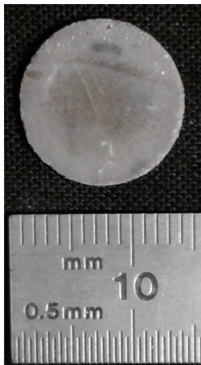
Figure 49. Darkened sample from sintering process
