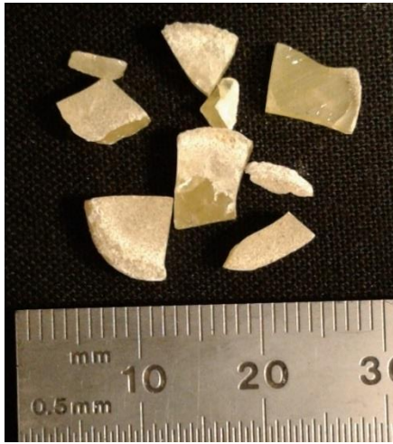
Figure 23. Photograph of sample 2 with top right piece polished on one side
