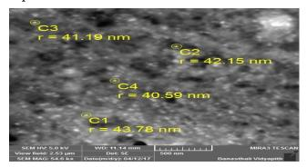
Fig. 9. SEM image of the synthesized nanoparticles
