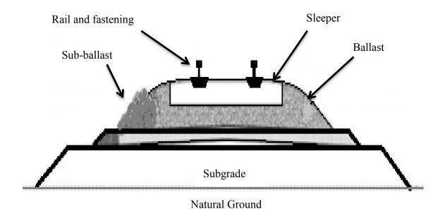
Figure 2.1: Cross-section of a single ballasted track on a fill (Bezgin, 2017)
