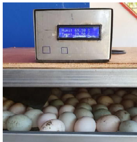
Figure 4. Control system in the hatching machine
