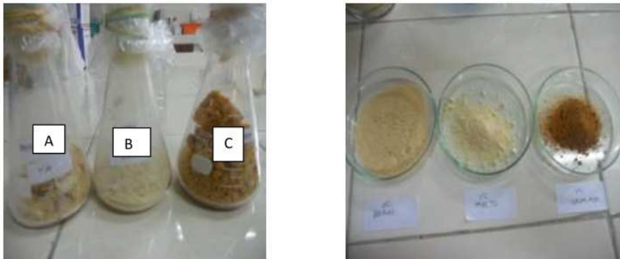
Figure 5. The effect of drying using various media on Color From Dry Culture, Rice Flour (A), Maltodextrin(B), Skim milk (C).
