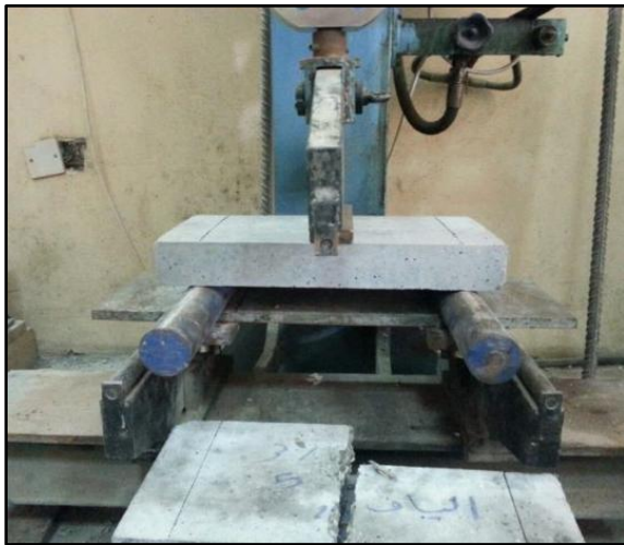
Figure 3. Flexural test of slab
