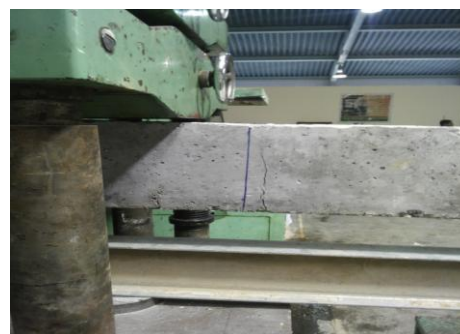
Plate 3. Beam flexural cracks
