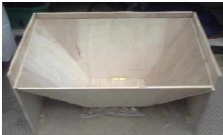
Figure 3. Truncated pyramid inserted into main solar oven cube
