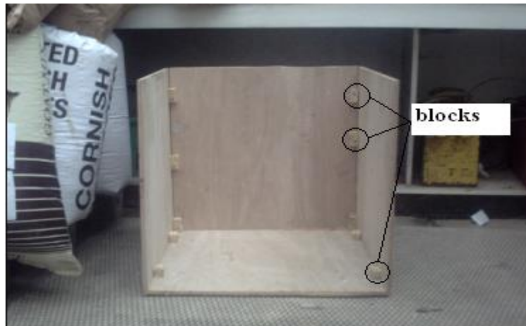
Figure 2. Joining blocks linking wood panels in the solar cooker
