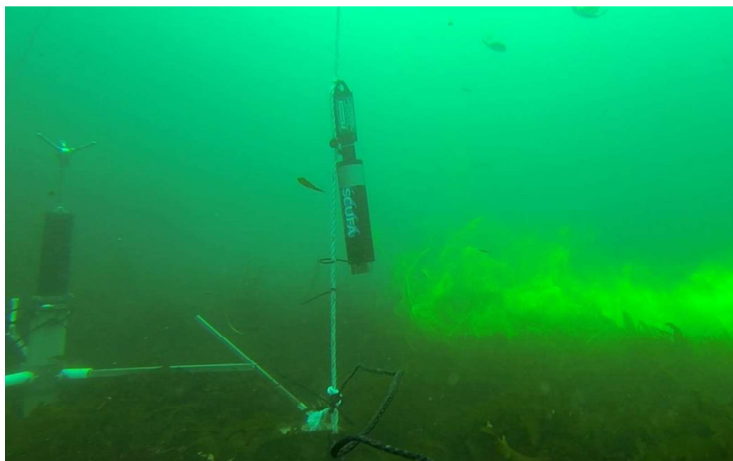
Figure 5: SCUFA (self-contained underwater fluorescence analyzer) array suspended through the water column. Three SCUFAs were placed at 1.5m intervals from the bottom and attached by line with an 8 lb. mushroom anchor and a surface float. The ADV (acoustic doppler velocimeter) was placed just downstream of the SCUFA array to not interfere with dye flow. The photo below shows the array set up outside of a kelp.
