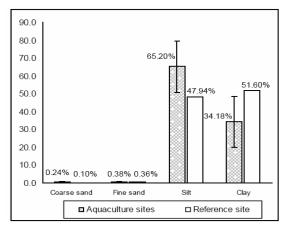
Fig. 5. Particle size composition of river sediment
