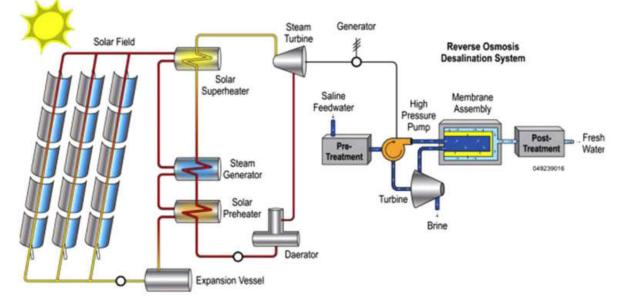
Figure 1. Schematic diagram of the Rankine cycle with solar field powering RO desalination system [8]
