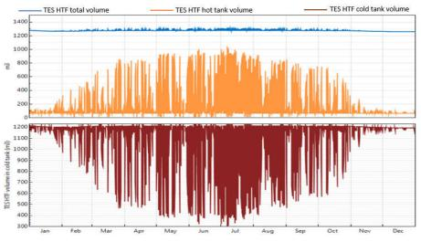
Figure 10. TES HTF total volume, hot and cold tanks volume
