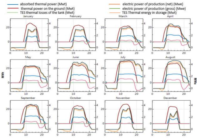
Figure 9. Absorbed thermal power (Mwt) and field power (Mwt), gross and net electric power (Mwe), TES thermal losses from the tank (Mwt) and in storage (Mwt)
