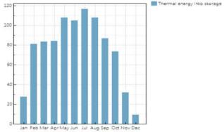
Figure 7. Monthly energy generated and thermal energy in storage (MWh)
