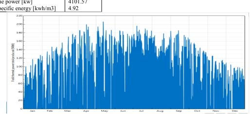
Figure 5. Total thermal power produced during the year (MWt)
