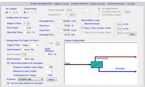
Figure 2. The configuration of the reverse osmosis system on ROSA
