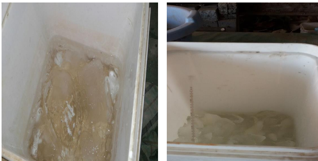
Fig. 1. Crushed ice used for cooling mixing water.
