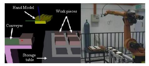
Figure 5: Virtual objects and actual laboratory set-up
