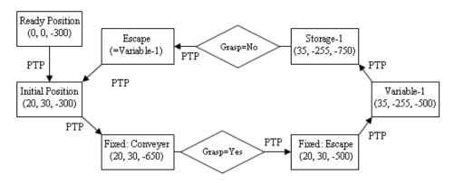
Figure 10: Complete path for the first work-piece.
