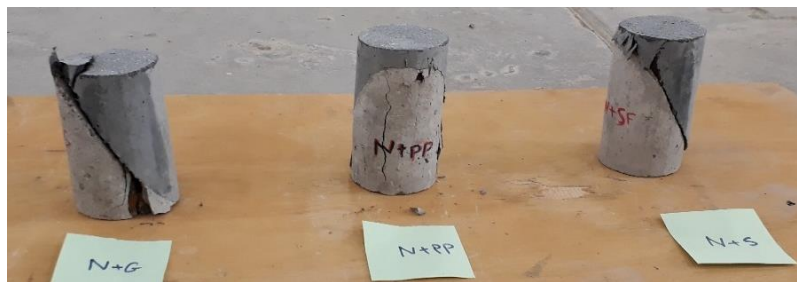
Figure 6. Slant shear failure for NSC with SF,GF and PPF
