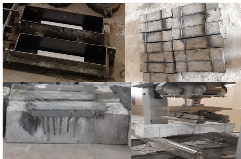
Figure 3. Preparation and testing specimen of composite prisms
