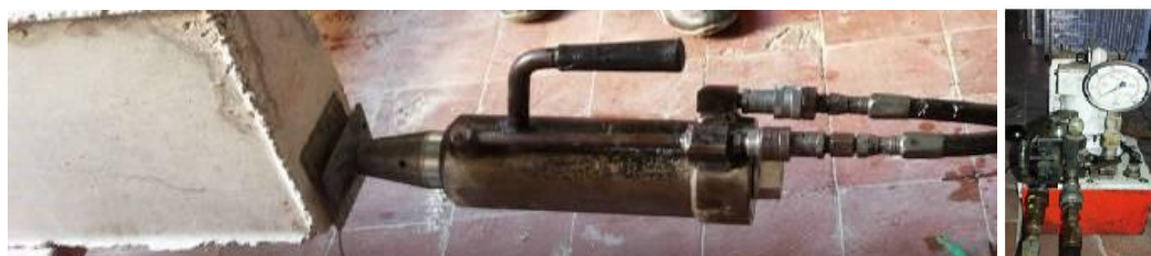
Figure 8. Jack pump and jack during tensioning
