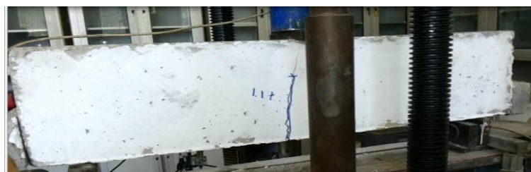
Figure 17. Crack Pattern and Mode of Failure of the fully prestressed beam without CNT after under temperature (FP – 400)
