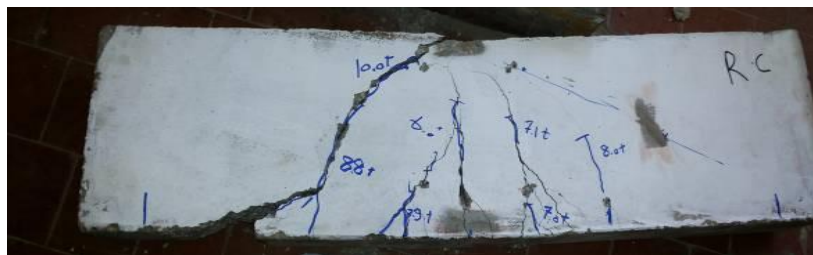
Figure 11. Crack pattern and mode of failure of a non-prestressed beam without CNT
