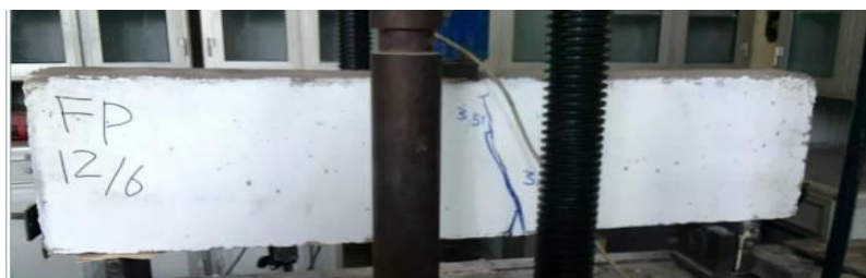
Figure 13. Crack pattern and mode of failure of the fully prestressed beam without CNT (FP)
