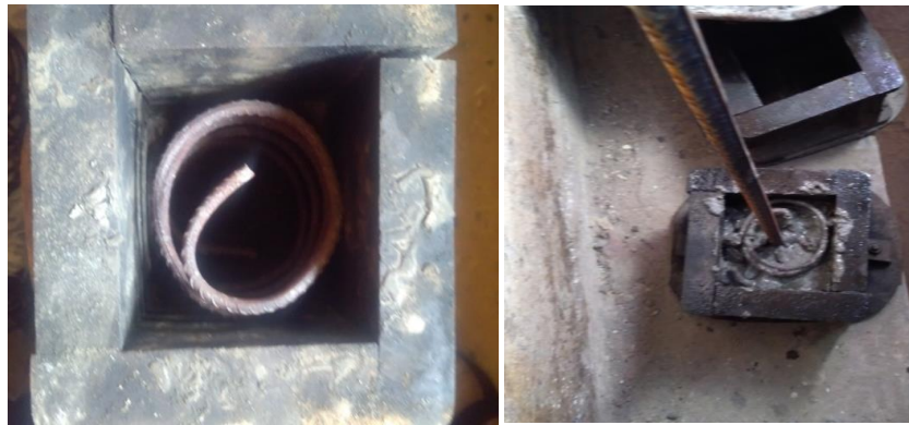
Figure 5. Helical reinforcement kept in position while casting
