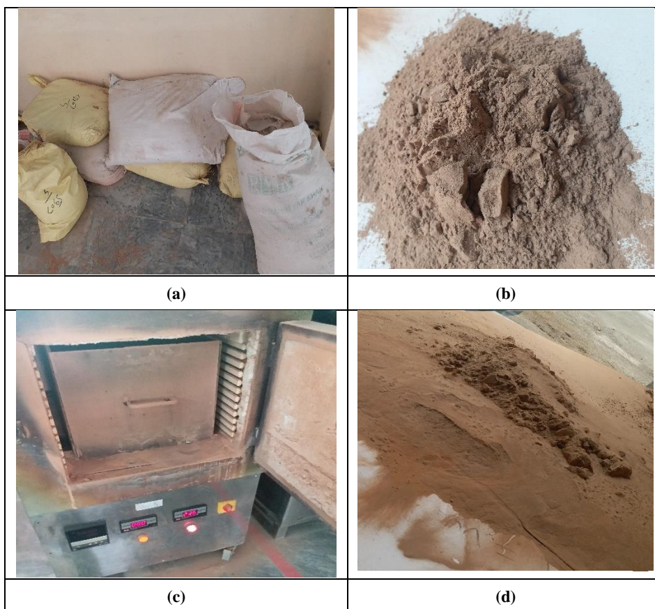
Figure 3. Montmorillonite used in the Research, (a) Mmt clay Received after grinding; (b) “As is” Mmt clay; (c) Heating of Mmt clay; (d) “Calcined” (800°C) Mmt clay
