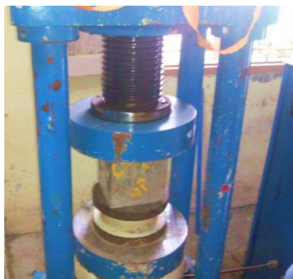
Figure 5. Compressive strength set up for cube
