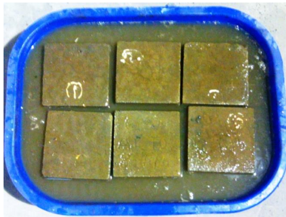
Figure 6. Cubes are immersed in HCL Solution
