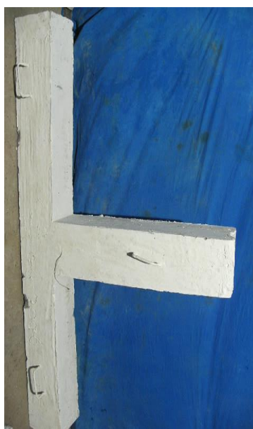
Figure 9. Typical beam – column Joint specimen ready for testing
