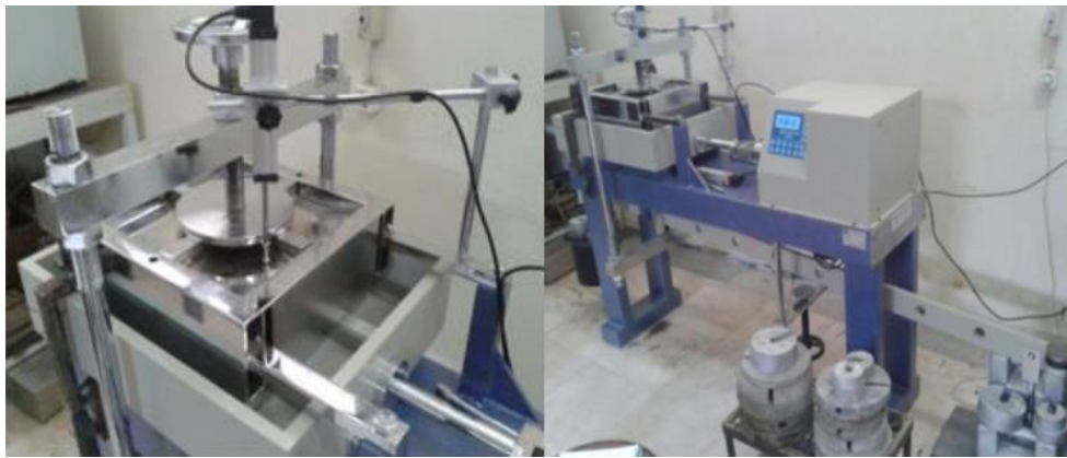
Figure 3. Large direct shear test apparatus used in this study [37]
