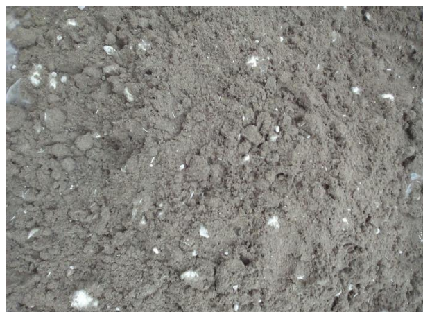
Figure 5. Fly ash-soil-cement mixture with 0.2% PVA fiber
