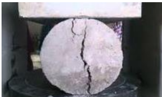
Figure 5. Cylinder in UTM under splitting tensile test setup
