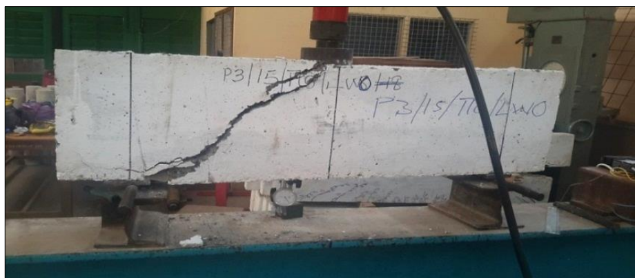
Figure 3. PKSC deep beam without shear reinforcement
