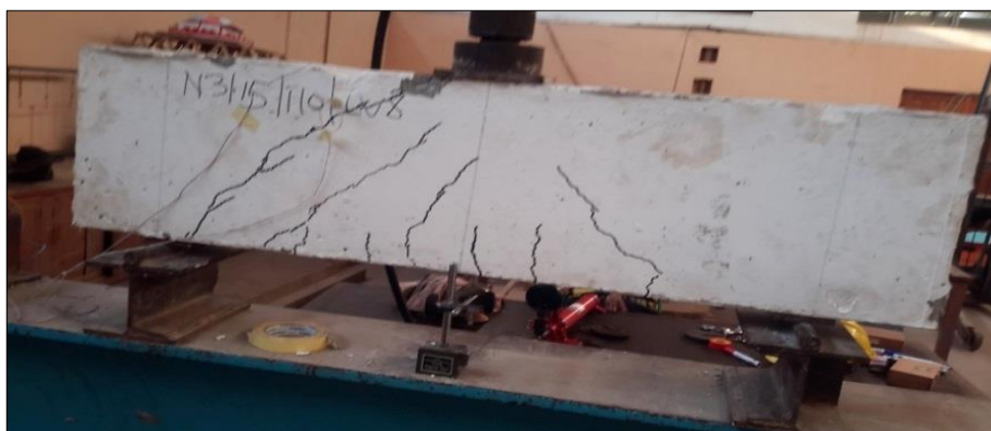
Figure 4. NWC deep beam with vertical shear reinforcement
