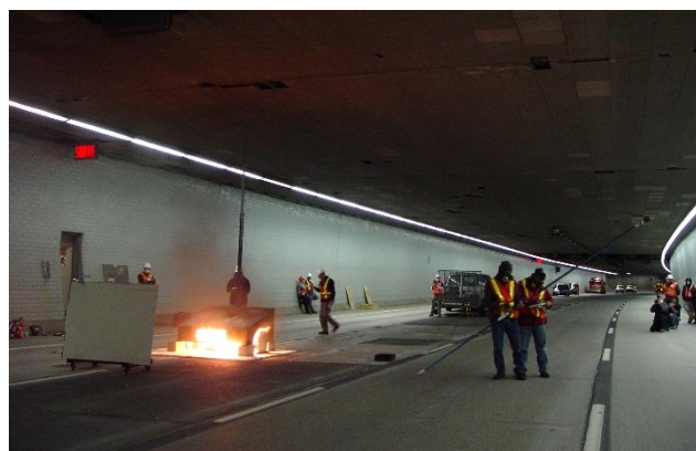
Figure 8. Fire tests in the Carré-Viger tunnel in Montreal, Canada [32]
