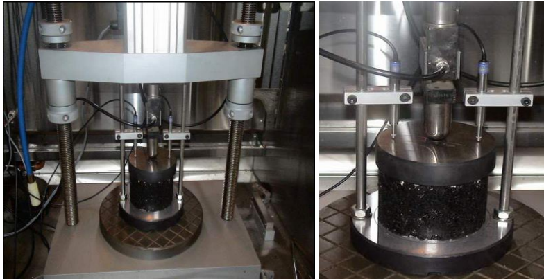
Figure 6. Dynamic creep test setup
