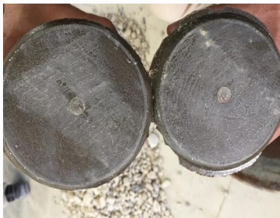
Figure 5. Two-headed two-way footpads for preparation to be placed under the Concrete breaker
