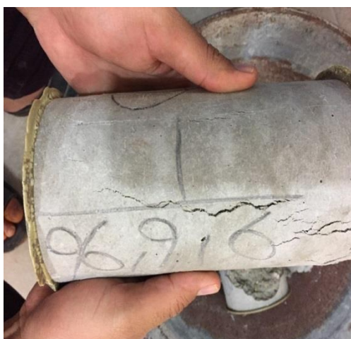
Figure 7. Broken sample after testing the compressive strength and how to create a crack in the sample
