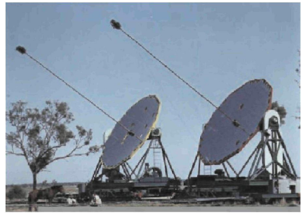
FIGURE 3. The two telescopes of the Intensity Interferometer in operation in Narrabri Australia until 1971.
